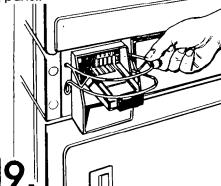
Insert top of wire guard Into holes on each side of the coin slide mechanism. Insert screws through hooked ends of guard and tighten. Repeat for other wire guard.
